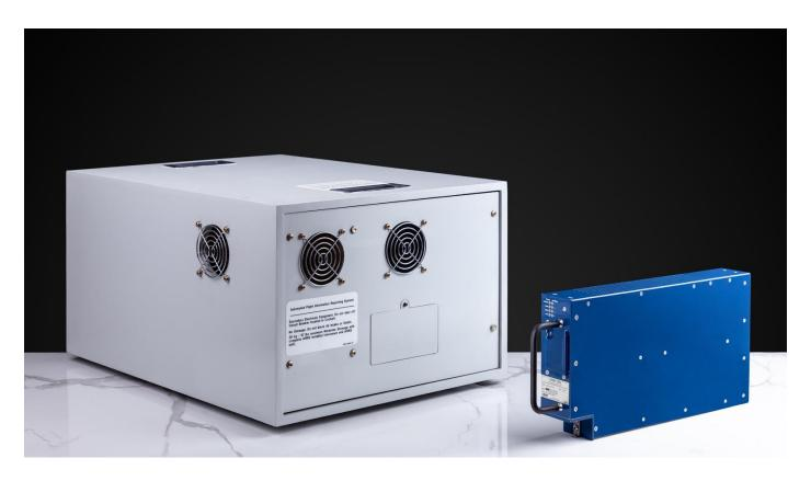
The first AFIRS prototype from 2002 (left) is shown versus the AFIRS 228 product that FLYHT markets today. The AFIRS 228 is the third production generation of AFIRS. The prototype shown here was installed in a Bombardier DHC-8 for approximately one year to collect data to guide the development of the first production AFIRS. FLYHT is celebrating 20 years as a company dedicated to improving aviation safety, efficiency and profitability.
